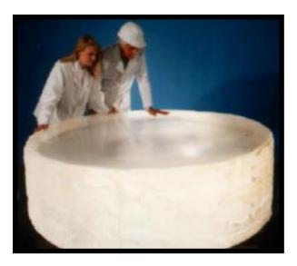
GE Quartz is a world leader in providing high purity fused quartz solid shapes for fabricators of quartzware. The solid shapes are available in three standard material types, each with various purity levels.
